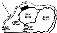
From Oman's History of the Art of War , by permission of Methuen & Co FIG. 3.—Berkeley Castle, late Norman Shell-Keep
